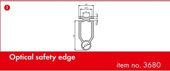
If the safety edge attached to the boom hits an obstacle during the closing procedure, the barrier stops and opens completely.
