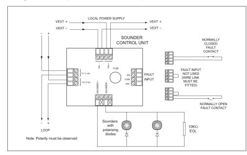
Fuse: 1.0A, anti-surge Local supply: 24V (9-32V) Sounder zone end-of-line resistor: 10KQ, 1/2Watt
