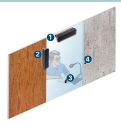
The loudspeaker must be mounted at least 1 m / 40 inches away from the microphone. If possible, the loudspeaker should not face the microphone directly because this leads to an echo of the operator voice at the inside station.
