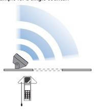
In this setup the speech of the operator is audible in the entire area in front of the counter.
